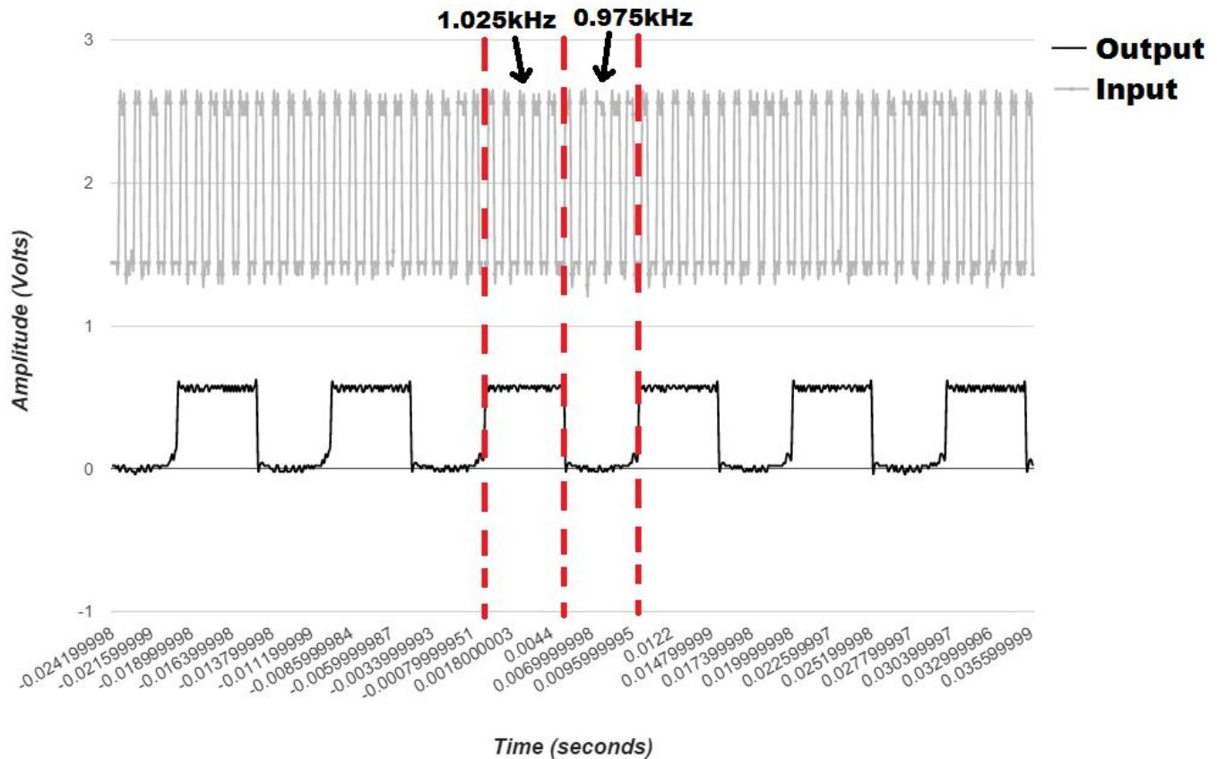
**Figure 2. Oscilloscope plot of input and output of FSK demodulator circuit showing TTL-compatible output switching between MARK and SPACE depending on input frequency. Some bit periods are highlighted to show how the output changes depending on input frequency.**
