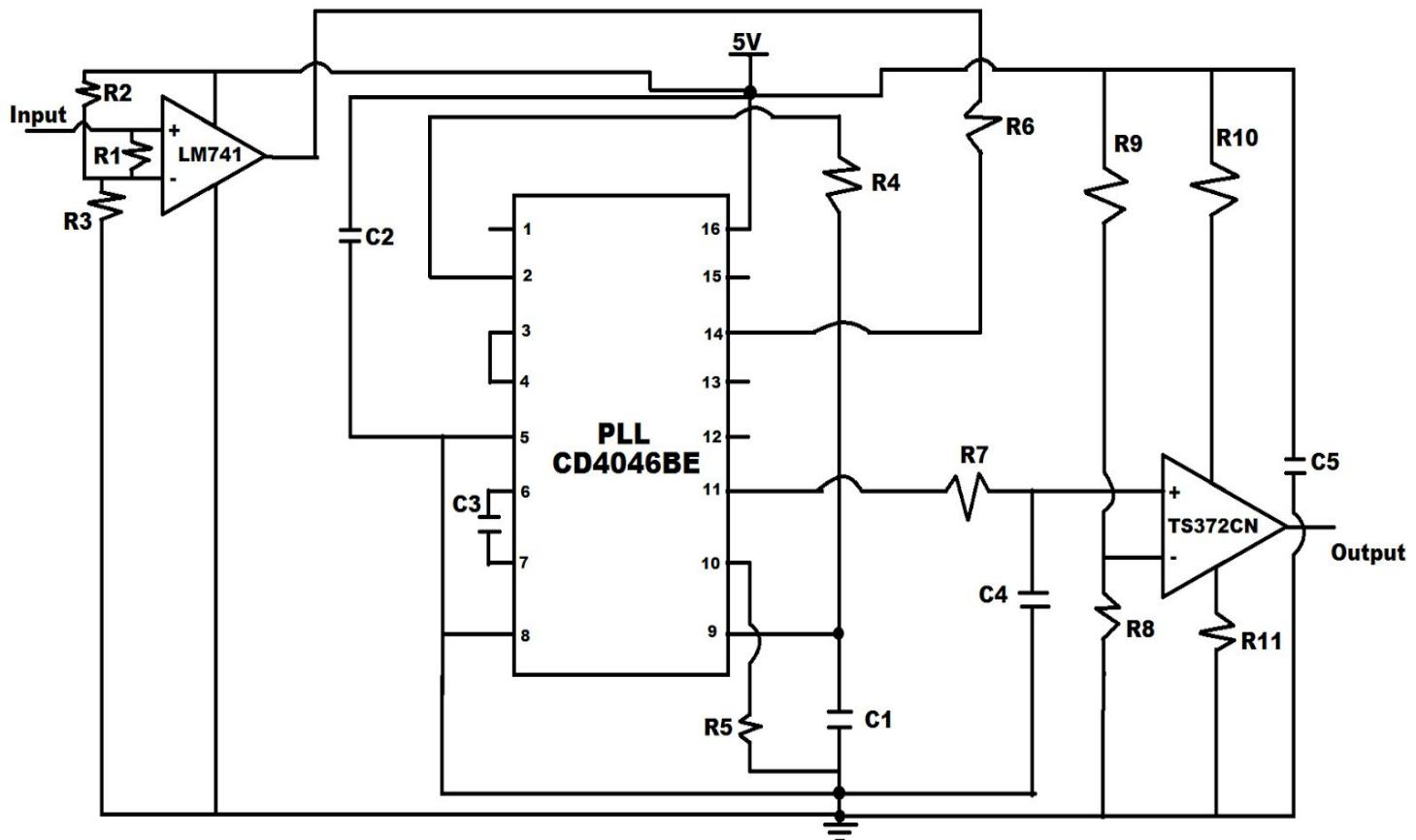
**Figure 1. PLL FSK demodulator circuit using the LM741 IC for the amplification stage, the CD4046BE IC for the PLL stage, and the TS372 IC for the comparator stage.**
